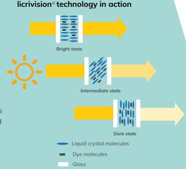
When a low voltage is applied, the dye-doped liquid crystals in the  $eyrise^{TM}$  cell change orientation and thus regulate the amount of light and heat passing through.
